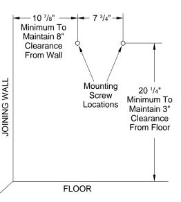
Figure 5 - Mounting Screw Locations
